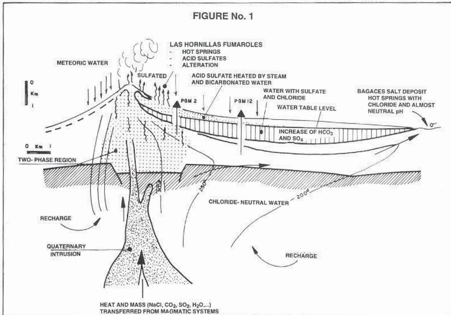
Conceptual model of the Miravalles Geothermal Field in Costa Rica. Example of a geothermal system associated with a volcanic apparatus (from Grigsby and others, 1989; adapted in Henley and Ellis, 1983). The Las Hornillas fumaroles are located over the hottest part of the reservoir, whereas the Bagaces Salt Deposit hot springs are found in the system's discharge zone.
