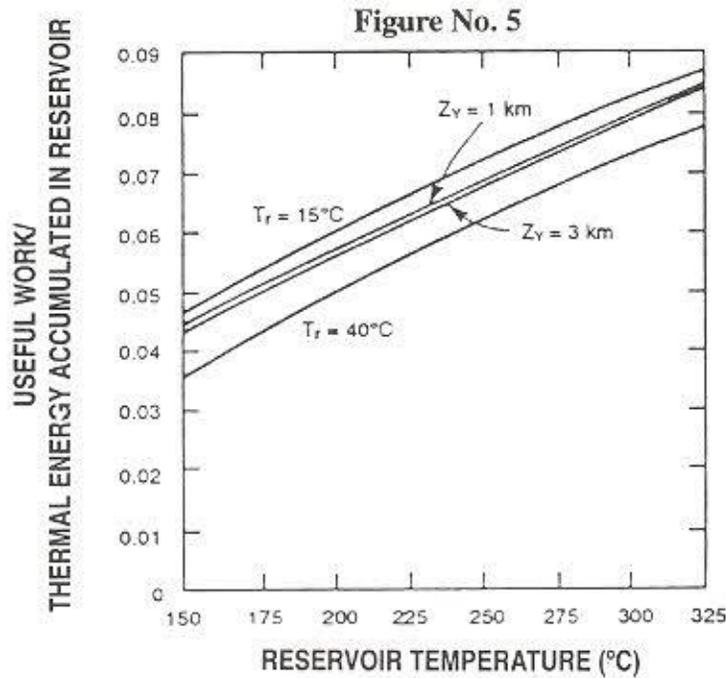
Ratio of Useful Work ( $W_u$ ) and Energy Accumulated in the Reservoir ( $q_Y$ ) versus Temperature, for geothermal systems of the liquid-dominated type. Two curves correspond to different average reservoir depths ( $Z_Y$ , from Brook et al., 1979) and another two to the different reference temperatures ( $T_r$ , from Paolo Liguori, personal correspondence, 1993). A Geothermal Recovery Factor of 0.25 was used to calculate  $W_u$ .
