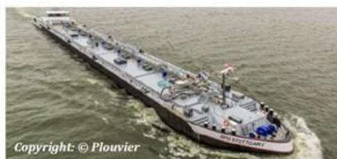
**Vessel type:** LNG-fuelled type C tanker
