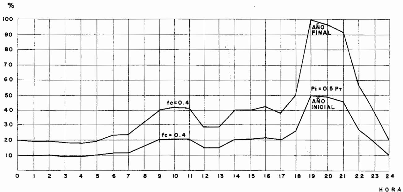
DIAGRAMA DE CARGA DE LA TURBINA PARA UN SISTEMA ELECTRICO CON  $f_c = 0.4$
