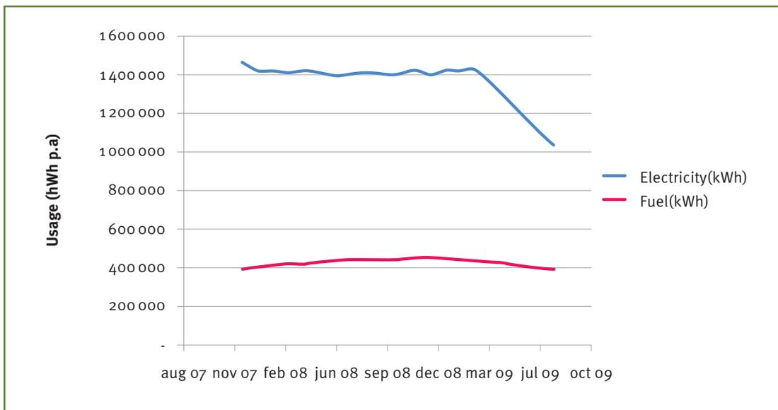
The trend in figure VII shows the same data but on an annualized basis, i.e. each point on the trend is the total of the previous 12 monthly bills. This view of the same data allows you to see overall trends of usage and is very useful for forecasting and budgeting usage.
