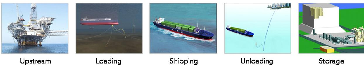
As a result CNG is expected to offer a lower cost gas transportation option than LNG for smaller volumes of gas over shorter distances (<1,500 – 2000 nautical miles), with easier and quicker permitting and implementation. CNG also has the added benefit that the majority of investment will be in the ships, which will be able to be redeployed to other projects as required.
