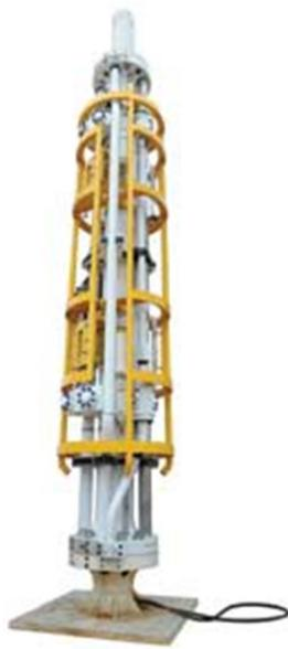
The figure above shows a subsea rotating control device (SRD) being shop tested in preparation of subsea mud-lift DGD application in the GoM.
