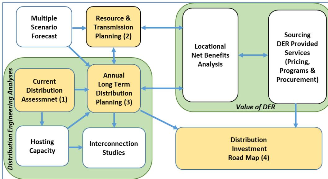
Figure 60 Integrated Distribution Planning Process
