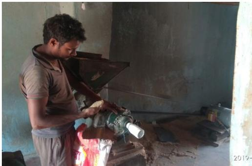
Two existing diesel-based rice hullers in Sahitoli were converted to electric and one new entrepreneur has bought an electric rice huller as an additional source of income since the conception of the mini-grid. Sahitoli was part of the Phase 1 and Phase 2 of the project which involved setting up mini-grids in eight villages.
